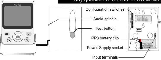
1. Move Key 13 to the right. Connect a 9V Alkaline PP3 to the battery clip.
